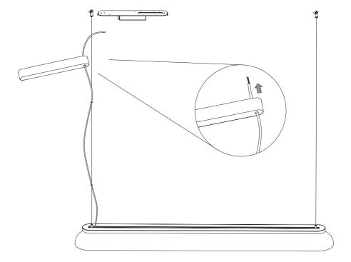
To secure the cable to the mounting bracket, start by loosening the screws on the cable clamps that are mounted on the mounting bracket, and pass the cable through. Once the cable is in place, tighten the screws again.
