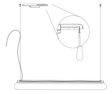
Pull the cable through the ceiling cap before connecting the cable to the driver.
