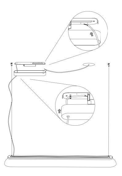
Fix the ceiling cap to the bracket using the provided screws.
