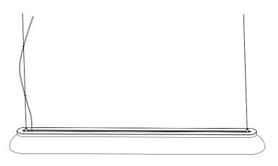
Lamp with suspension wire & cable
