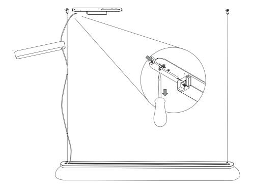
Wiring to mains power: Taking one wire at at a time, insert the correct wires into the corresponding slots on the terminal block, while pressing down on the small button next to them. The live mains wire should be inserted into the slot marked L and the neutral mains wire into the slot marked N. If you are unsure of the polarity of the wires, then we recommend you contact a certified electrician.
