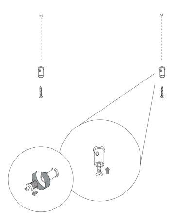
Once the suspension mounts are firmly in place, the lamp is ready to be mounted. Start by pulling the suspension wire through the disassembled suspension mount (step 1). Guide the wire though the fixed suspension mount and through the exit hole on the side (step 2). Screw the disassembled suspension mount together with the part that is fixed to the ceiling (step 3). The suspension wire is now safely in place (step 4). Repeat on the other side.
