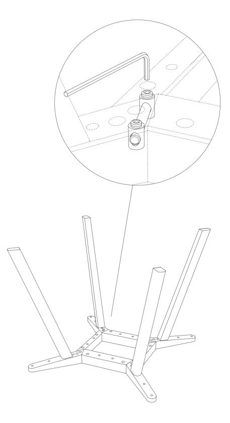
Use 4 of the F parts for perfect alignment. Screw them lightly in the hole, but don't tighten them completely.
