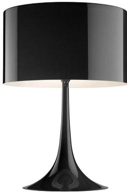
Table/desk lamp providing diffused light. Spun metal frame and diffuser, die-cast aluminum diffuser support arms and lampholder support, painted in the colors indicated below. White, injection-molded polycarbonate diffuser supports. Sandblasted pressed glass upper diffuser screen. On the cable there is the electronic dimmer which allows the regulation of light brightness.
